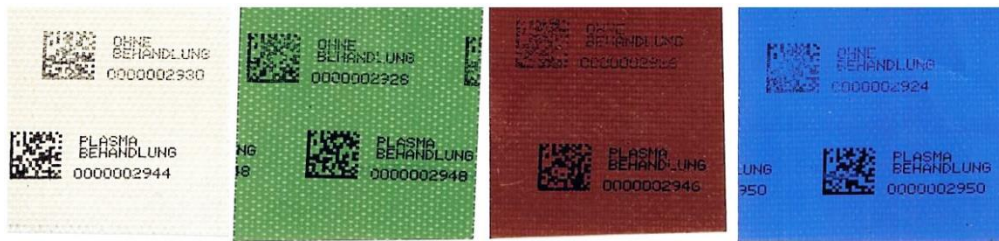
Figure 4: Comparison of print image without plasma pre-treatment (top) and after plasma treatment (bottom)
