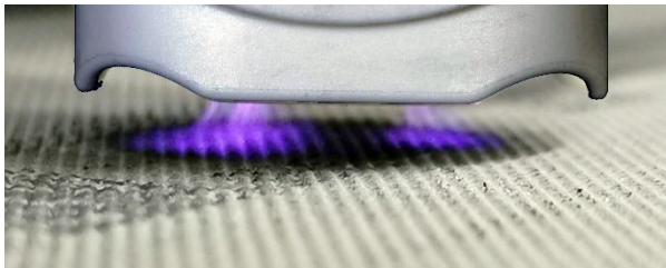
Figure 2: Plasma treatment with PiezoBrush PZ3-i
