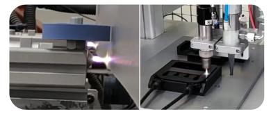
There are three different nozzles for the PlasmaBrush PB3 system, which are optimised for low-potential processes, sensitive materials and high process speeds.
